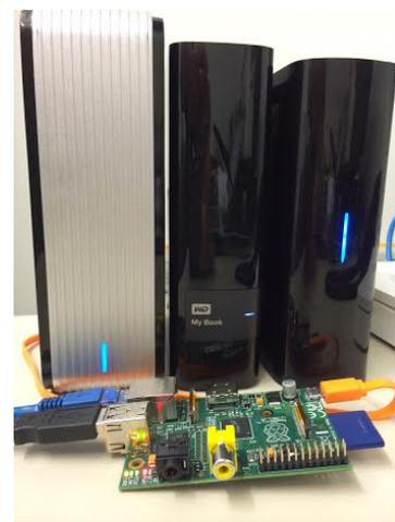
Figure 1. FixityBerry, which includes a Raspberry Pi connected to USB hard drives.
